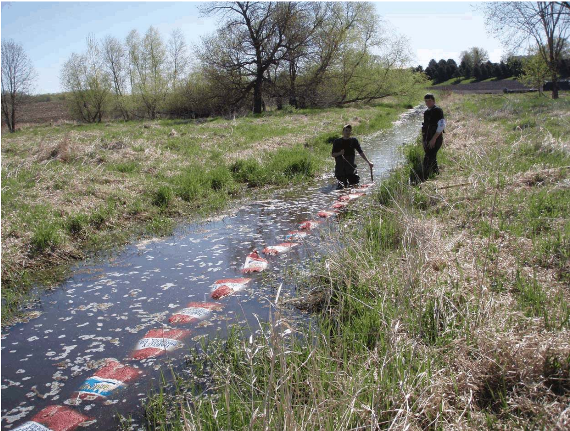
Figure 1. On May 14, 2008, barley straw was added to the stream that outflows a ditched wetland that flows into Lake Volney.
